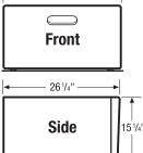
For built-in installations, NO minimum clearance required around sides or backs of units. For closet installation, allow additional 1" clearance between fronts of units and door, Location of plumbing, exhaust and utility hookups MUST be considered in built-in installations. For additional installation details, refer to Product Installation Guides on web
